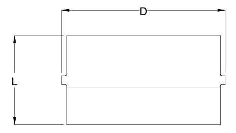
Fittings between 20" and 48" are designed to be fused on a 1648 or smaller field machine, If longer lengths are required, please contact Sandale Utility Products for special requirements.
