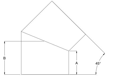
Fittings between 20" and 48" are designed to be fused on a 1648 or smaller field machine, If longer lengths are required, please contact Sandale Utility Products for special requirements.
