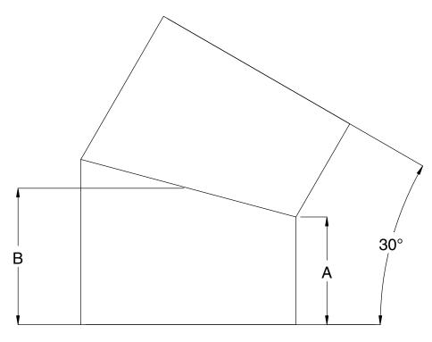
Fittings between 20" and 48" are designed to be fused on a 1648 or smaller field machine, If longer lengths are required, please contact Sandale Utility Products for special requirements.
